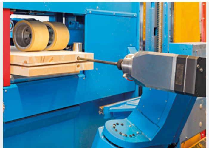
For special applications, drills of up to d=50 mm and an effective length of 420 mm can be used
