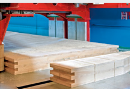
26 Saw cut with splitting
