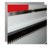
The tables on the right and left finger shapers move on precision linear quide ways in combination with rack/pinion transmission for extra smooth movement
